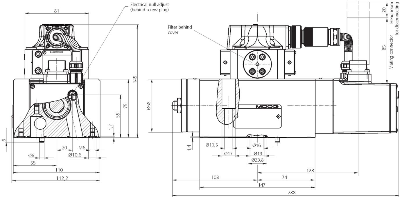
The mounting manifold must conform to ISO 10372-06-05-0-92.
