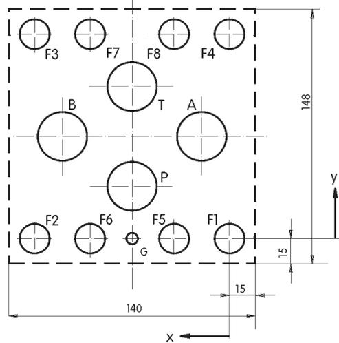
**Note:** The X and Y tubes have to be connected to the Moog valve body by fittings. Mounting surface needs to be flat within 0,02 mm. Average surface finish value, Ra, better than 1µm.
